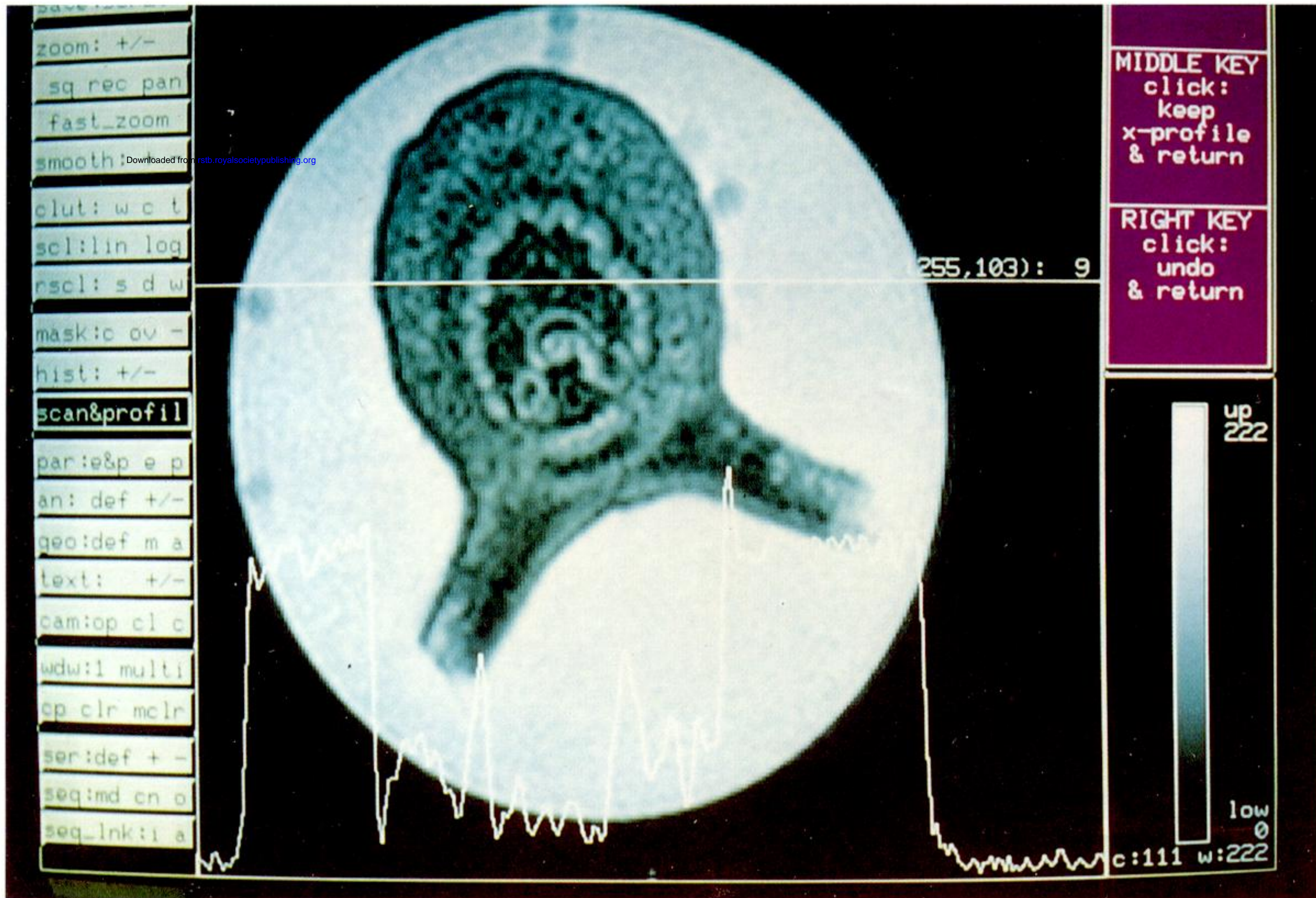
Figure 2. Typical ^1\text{H} -spin-echo NMR image and signal intensity profile of a cross-section of an excised leaf of Argyroderendron calatum (Queensland, Australia, leaf cut at 32 m height). The tree had been subjected to prolonged drought. Experimental conditions were as in figure 1 (E. Kuchenbrod, A. Haase, R. Benkert, H. Schneider, G. Zimmermann & U. Zimmermann, unpublished data). It is evident that the signal intensity throughout the tissue is very low indicating the presence of a substantial amount of air and correspondingly a relatively low water content. Xylem pressure probe measurements confirmed this result (see figure 8).
